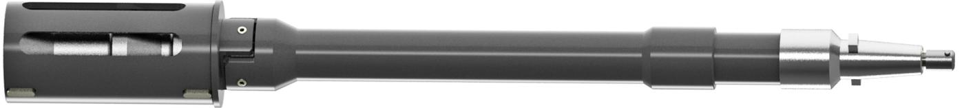
514-9D Hone Head Stone Holder Sets require 2 sets of 4 diamond stones - 3" (76mm) long Diamond stones. Total Length of Stone Holders 6" (152mm)
