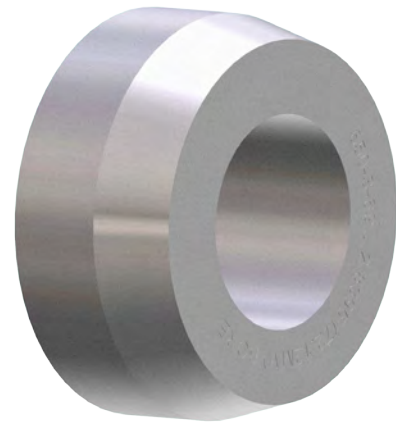
650-3-72A Locator - Main #1 (2.8504 - 2.8513" bore) (72.40 - 72.42mm)
