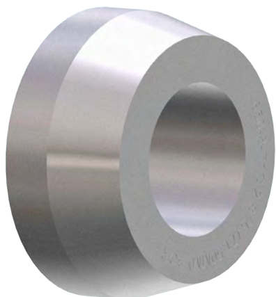
650-3-71C Locator - Main #1 (2.8150 - 2.8160" bore) (71.50 - 71.53mm)
