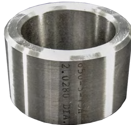
650-3-15H Locator, Cam (2.0292 - 2.0310" bore) (51.51 - 51.58mm)
