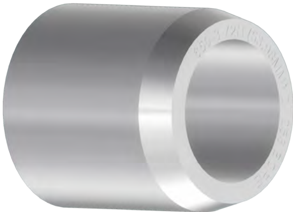
650-3-88C Locator - Main #5 (2.1440 - 2.1455" bore) (54.46 - 54.50mm)
