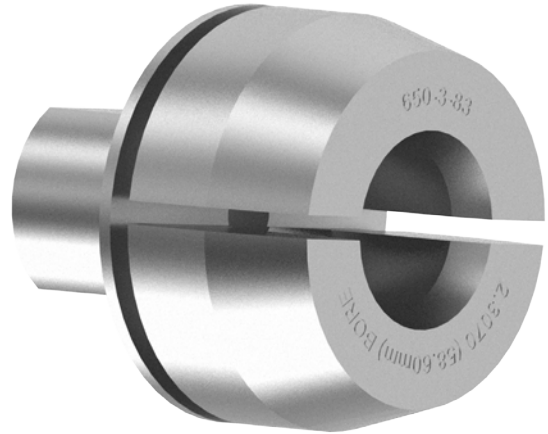
650-3-70J Locator, Cam, Expanding (2.3475 - 2.3490" bore) (59.60 - 59.66mm)
